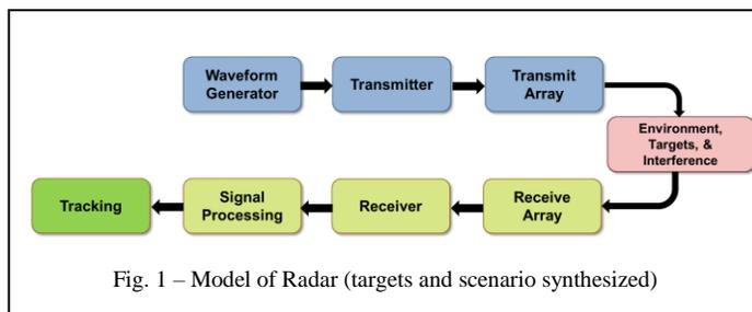
For the study, a commercially available phased array radar was used to generate processed data. This data was compared to simulated data generated with the models. The selected hardware implementation also provided a source of live data for algorithm development.
