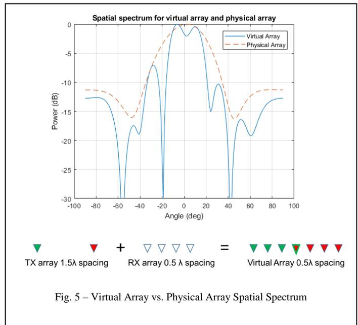
Fig. 5 – Virtual Array vs. Physical Array Spatial Spectrum
