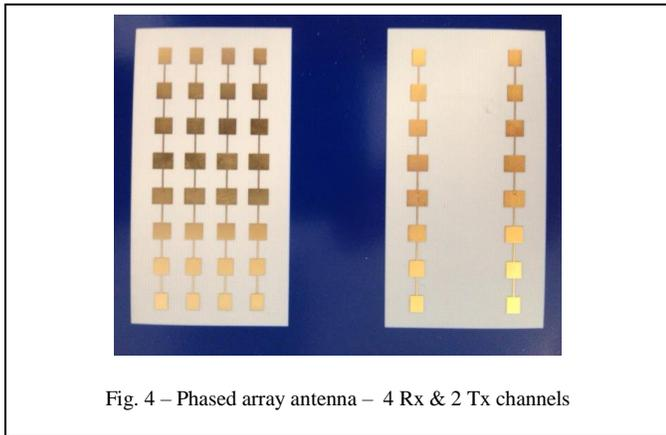
Fig. 4 – Phased array antenna – 4 Rx & 2 Tx channels
