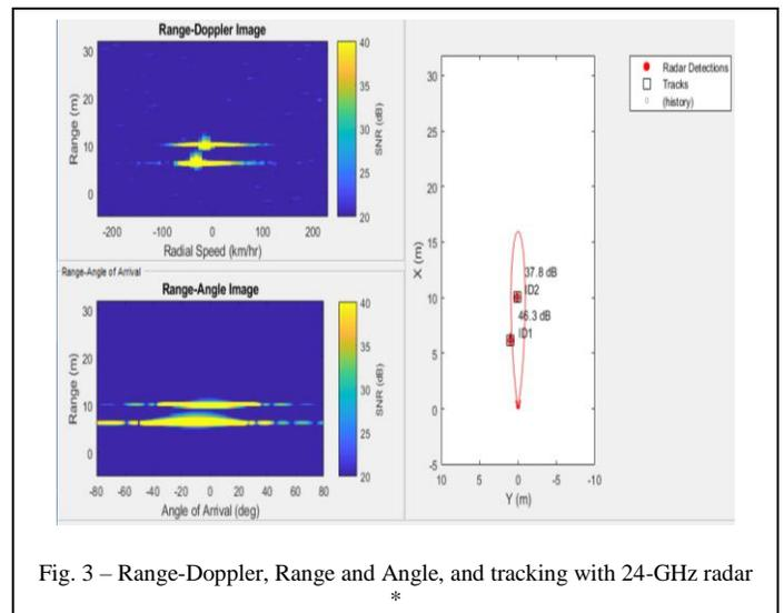
Fig. 3 – Range-Doppler, Range and Angle, and tracking with 24-GHz radar \*
