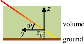
Fig. 4. Dual-layer forest model, consisting of a volume, which is a lossy propagation medium, above a ground surface at  $z = z_g$ , which is a hard propagation boundary. The model is assumed reasonable at L-band. The SAR images are focused to  $z = 0$ .
