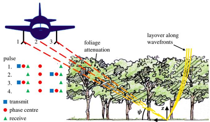
Fig. 1. Left: a dual-antenna, across-track interferometer that synthesises three effective phase centres separated in grazing angle  $\psi$  by alternating the transmit antenna pulse-to-pulse and receiving every pulse on both antennas. Right: canopy attenuation and layover.
