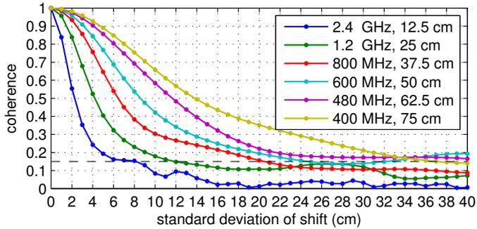
Fig. 3. Coherence magnitude at different wavelengths as a function of the level of change in a clutter scene. Each curve was obtained by repeated execution of a SAR simulation where change was implemented as random shifts in the positions of point scatterers. The resolution was fixed.
