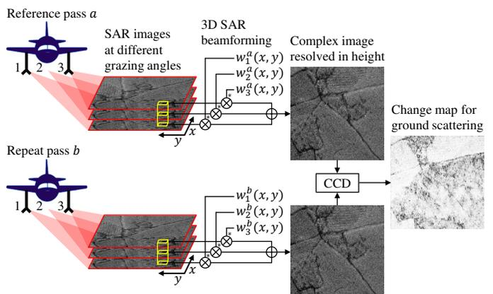
Fig. 2. The proposed 3D SAR CCD concept. SAR images from each pass of a multichannel radar system are vertically beamformed using complex weights  $\mathbf{w} = [w_1, w_2, \dots]^T$ , which may vary spatially, to produce a complex ‘3D’ image steered to the ground, with canopy scattering suppressed. The magnitude of the complex coherence between two 3D images indicates change at ground level.
