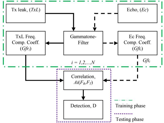
Fig. 4. Bio-inspired detection mechanism for human echo locator click signal
