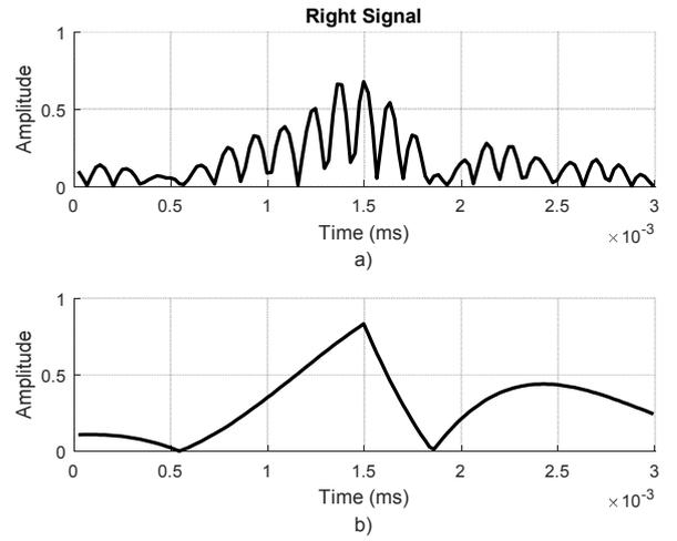
Fig. 6. Correlation of individual channels of Gammatone filter bank from the right signal, a) Output from highest channel order,  $i = 1$  (containing highest frequency component from EE waveform), b) Output from lowest channel order,  $i = 10$  (containing lowest frequency component from EE waveform)
