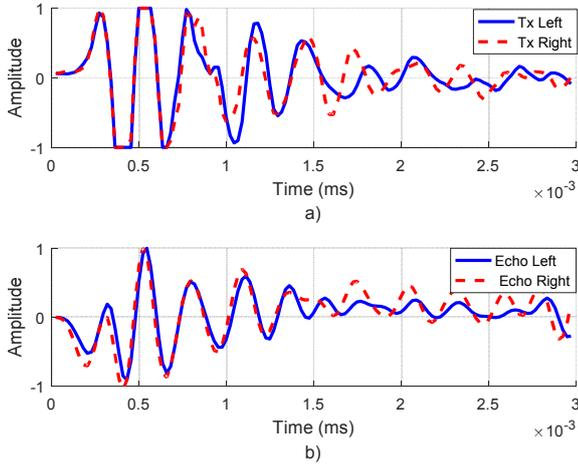
Fig. 2. Time domain of EE signal, a) Transmitted signal, b) Echo signal
