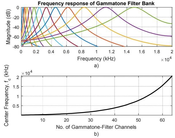
Fig.1. Characteristics of the Gammatone filter, a) Frequency response of Gammatone filter bank, b) Trend of individual channel widths in the Gammatone filter, which increases in the form of an logarithm factor
