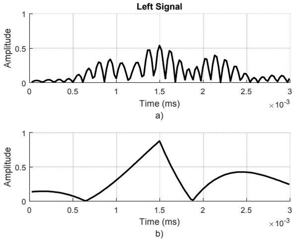
Fig. 5. Correlation of individual channels of Gammatone filter bank from the left signal, a) Output from highest channel order,  $i = 1$  (containing highest frequency component from EE waveform), b) Output from lowest channel order,  $i = 10$  (containing lowest frequency component from EE waveform)
