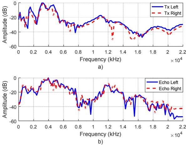
Fig. 3. Power Spectrum Density of EE signal, a) Transmitted signal, b) Echo signal
