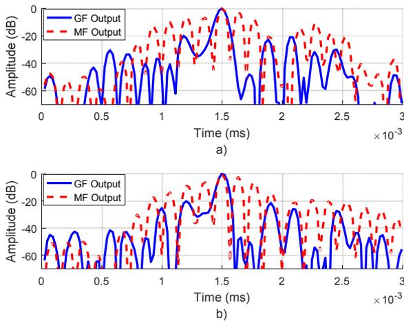
Fig. 8. Detection output between propose method (incorporated GF) and MF processing, a) Left signal, b) Right signal. The result is converted into a normalized representation in order to observe the cross-correlation level, which reflects the overall detection results
