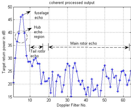
Fig. 6. Helicopter modulation in Doppler domain (Real data)
