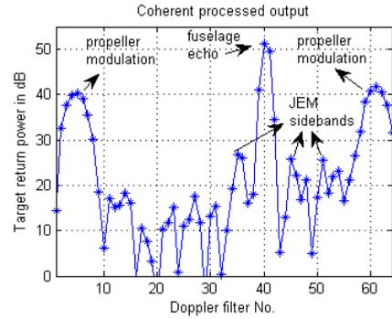
Fig. 5. JEM with propeller modulation in Doppler domain (Real data)
