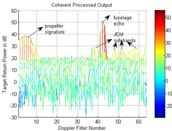
Fig. 4. JEM signature with propeller (Simulated)
