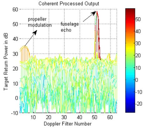
Fig. 2. Propeller aircraft signature (Simulated)
