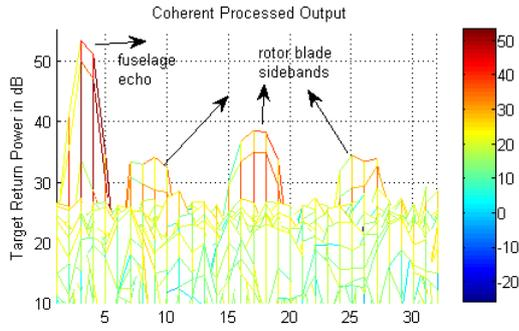
Fig. 3. Helicopter rotor engine modulation (Simulated)
