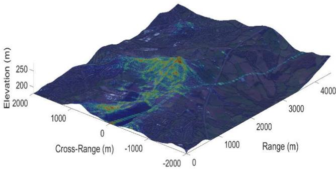
Fig. 6. Topographic map of the Bartley Reservoir area, overlaid with a satellite image of the area and the SAR image shown in fig. 5.
