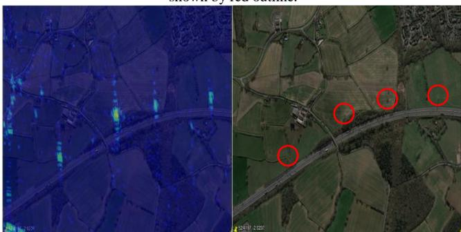
Fig. 9. Subsection of the SAR image shown in figure 5. (a) SAR image of an area around a series of electricity pylons, overlaid with a satellite image of the area. (b) Satellite image of the area shown in (a) electricity pylons highlighted by red circles.
