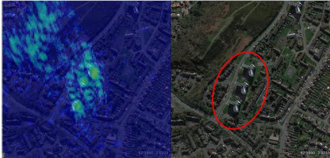
Fig. 7. Subsection of the SAR image shown in figure 5. (a) SAR image of an area surrounding three high-rise buildings (highlighted by red outline) overlaid with a satellite image of the area. (b) Satellite image of the area shown in (a).
