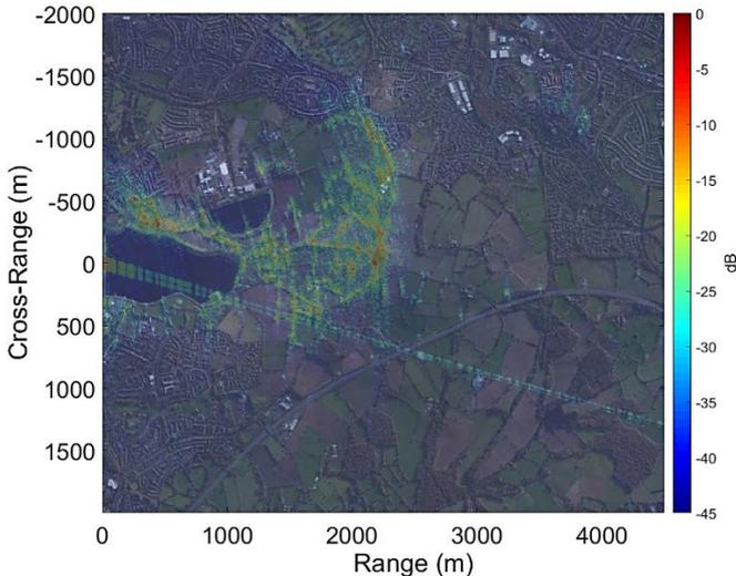
Fig. 5. Reconstructed SAR image of Bartley Reservoir target scene from road measurements, overlaid with ground-truth satellite imagery.
