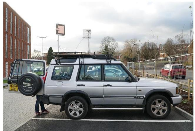
Fig. 3. Land Rover Discovery vehicle used for ground-based measurements, with two patch antennas mounted on 1.5 long poles atop the roof of the car.
