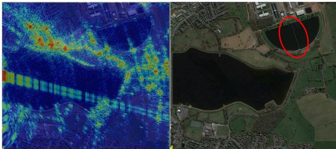
Fig. 8. Subsection of the SAR image shown in figure 5. (a) SAR image of an area around Bartley Reservoir overlaid with a satellite image of the area. (b) Satellite image of the area shown in (a) with walkway over smaller reservoir shown by red outline.
