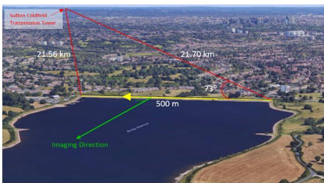
Fig. 2. Image of the Bartley Reservoir road, with the aperture track shown in yellow, the imaging direction in green, and the direction to the Sutton
