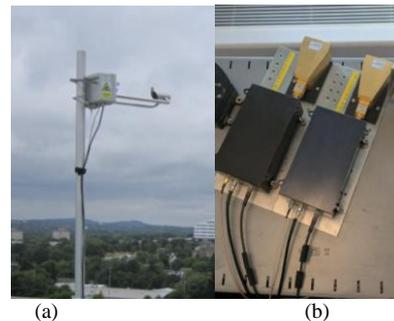
Figure 1. Measurement setup (a) laser precipitation monitor and (b) 300 GHz radar
