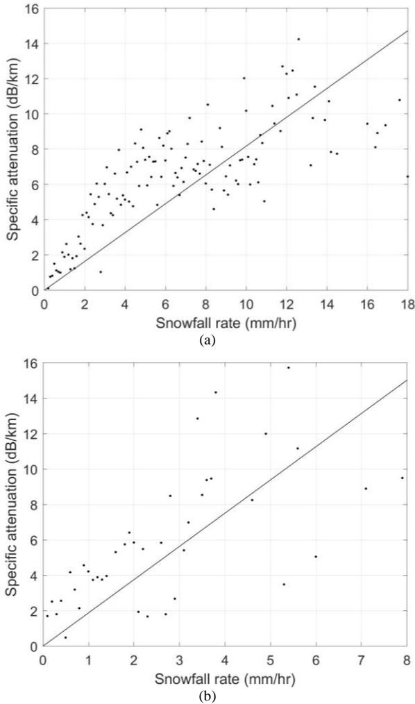
Figure 4. Measured specific attenuation at 300 GHz through (a) dry snow and (b) wet snow
