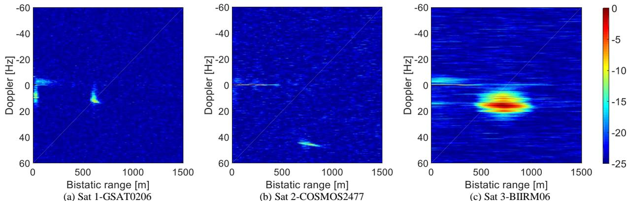
Fig. 4. Example RD maps of target from a) Galileo, b) GLONASS, c) GPS satellite.
