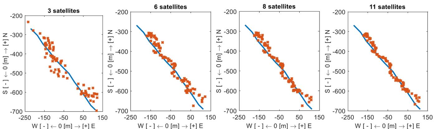
Fig. 5. Target location vs no. of satellites
