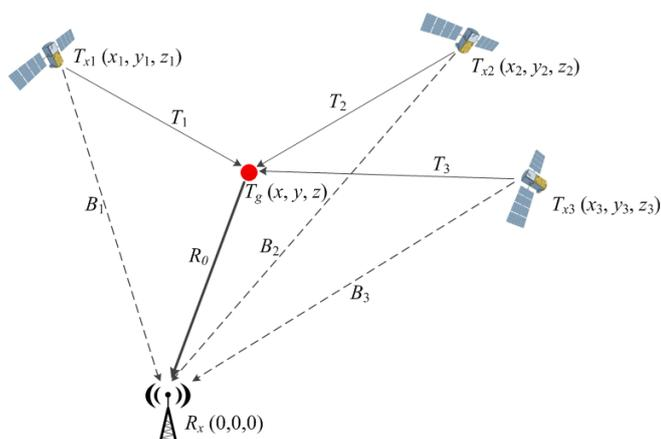
Fig. 1. Multistatic GNSS-based radar ( $N=3$  in this example).
