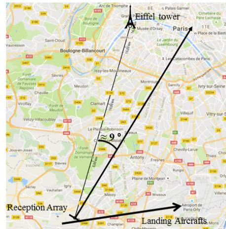
Fig. 7. Geometry for the experimental setting. The reception device is located in south of the Parisian suburban area, at a few kilometers west from the Orly airport. The transmitter (Eiffel tower) is located in a direction of approximately 9 with respect to the normal of the reception array. Aircrafts landing at the Orly airport pass in the South near the reception device.
