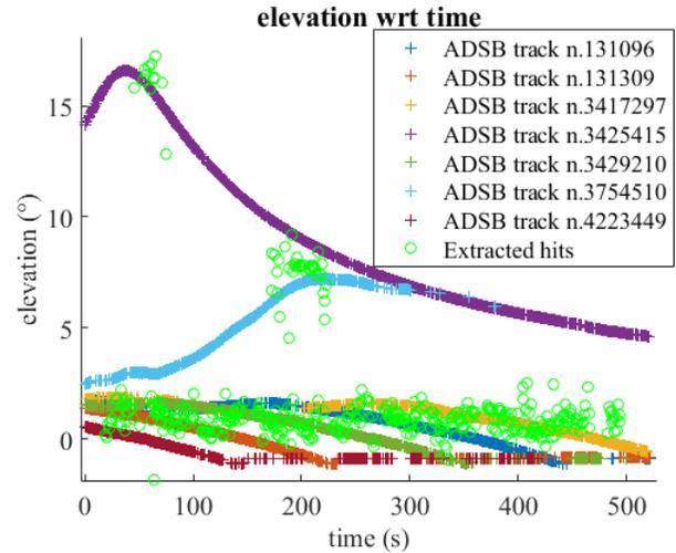
Fig. 10. Evolution of the target elevation with respect to time, as provided by the ADSB measurements, and corresponding extracted hits estimated from the MIMO-FM processing. The elevation estimation presents a relatively high variance, but clearly the MIMO-FM processing enabled to discriminate targets landing at Orly airport from other targets flying higher.
