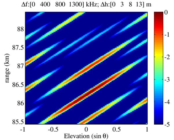
Fig. 5. Ambiguity function for  $N_T = 4$  transmitters located at heights [291, 294, 299, 304] m, and transmitting respective frequencies [101.9, 102.3, 102.8, 103.3] MHz. The target is present at range 86.22 km and elevation 0. The range domain considered corresponds to the range cell of the target.
