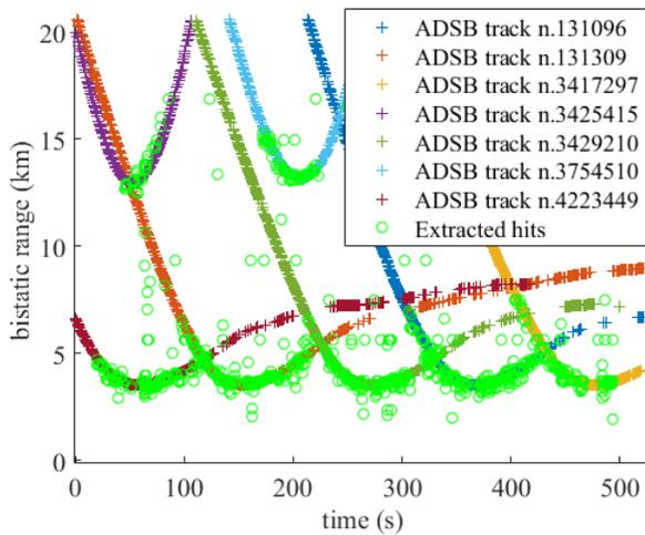
Fig. 9. Evolution of the target range with respect to time, as provided by the ADSB measurements, and corresponding extracted hits estimated from the classic FM processing. In that case, the range estimation is worse than in the MIMO-FM case (see Figure 11), which is expected since only one subband with small bandwidth is used for the estimation.
