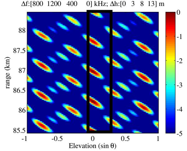
Fig. 4. Ambiguity function for  $N_T = 4$  transmitters located at heights [291, 294, 299, 304] m, and transmitting respective frequencies [102.7, 103.1, 102.3, 101.9] MHz. The target is present at range 86.22 km and elevation 0. The range domain considered corresponds to the range cell of the target. The black rectangle represents the domain of interest, i.e. low altitude targets.
