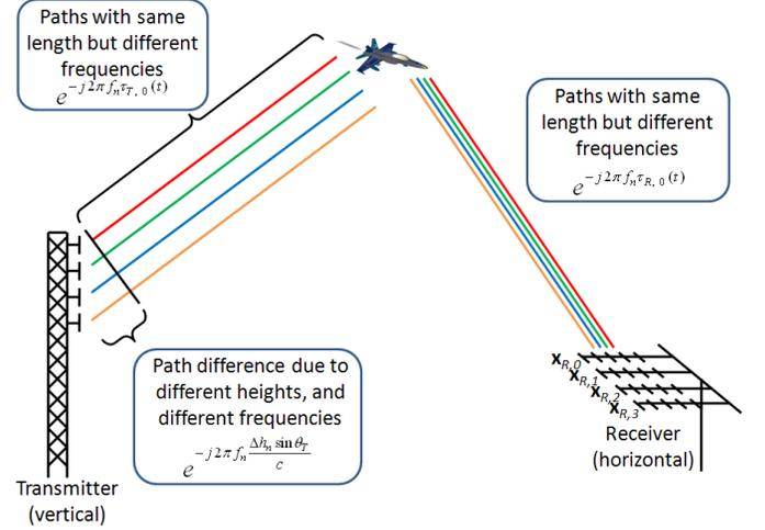
Fig. 2. Geometric configuration for the MIMO-FM passive radar. Since the path difference at the reception side is due to the horizontal positions of the different receiving antennas, it does not impact the elevation estimation and was not represented here.
