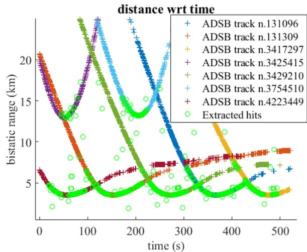
Fig. 11. Evolution of the target range with respect to time, as provided by the ADSB measurements, and corresponding extracted hits estimated from the MIMO-FM processing. The range parameter is very accurately estimated, taking benefit from the overall MIMO-FM bandwidth.
