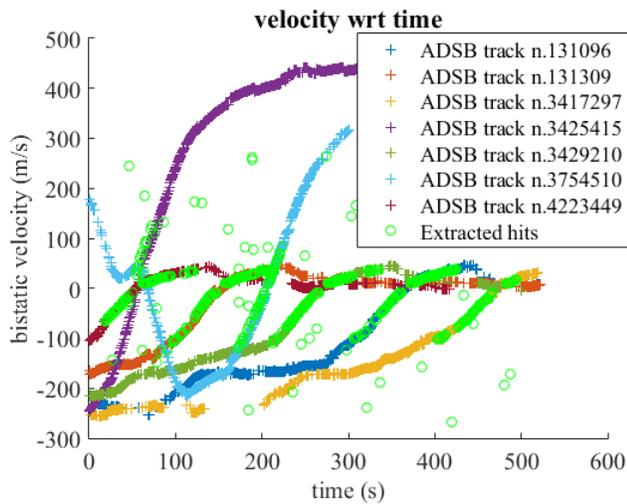
Fig. 8. Evolution of the target velocity with respect to time, as provided by the ADSB measurements, and corresponding extracted hits estimated from the MIMO-FM processing.
