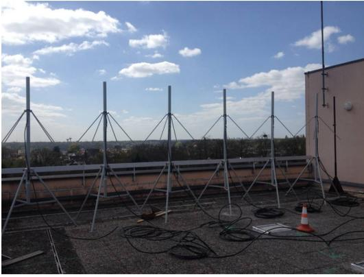
Fig. 6. Reception device of the experimental setting. Although the reception array was composed of six antennas, only four were used for the processing.
