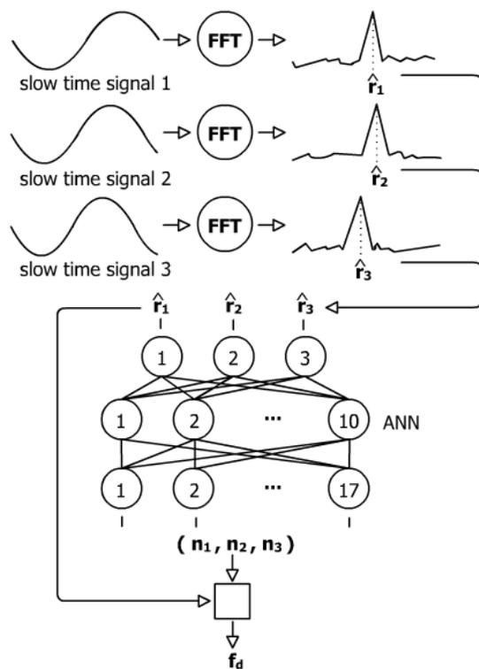
Figure 1: Overview of the method to determine the Doppler frequency using ANN
