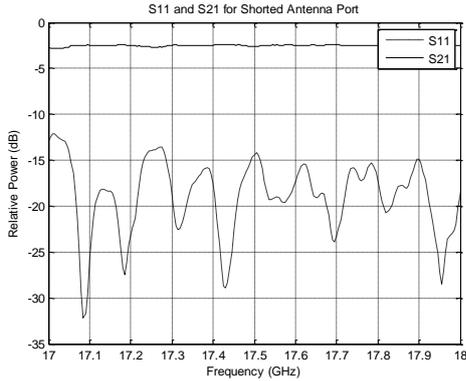
Fig. 7. Measured return (S11) and transmission (S21) losses for the waveguide sections of the RASS with minimal contribution from the RPC
