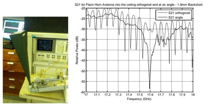
Fig. 9. Photograph of the RASS with the standard gain horn antenna and return loss tuned to 17.6 GHz with the beam perpendicular to the ceiling and at an angle
