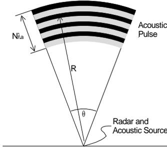
Fig. 2. RASS geometry illustrating the focus effect of collocated sensors
