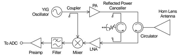
Fig. 3. Schematic diagram of the Doppler radar and reflected power canceller
