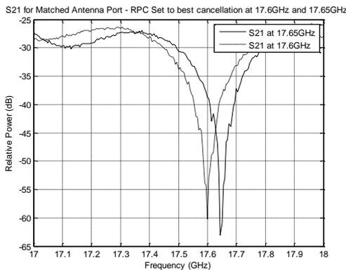
Fig. 8. Measured transmission losses for the waveguide sections of the RASS with the RPC adjusted for maximum cancellation at 17.6 and 17.65 GHz
