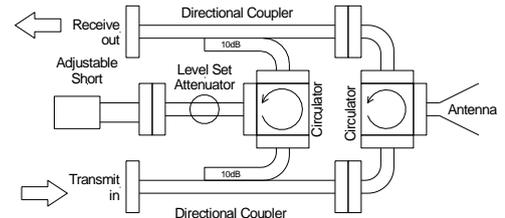
Fig. 6. Block diagram of the waveguide components of the Doppler radar portion of the RASS
