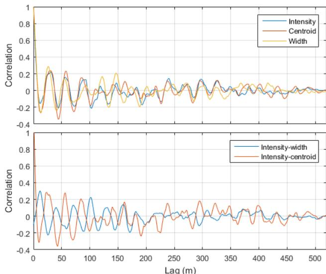
Fig. 4. (Top) Range autocorrelation of the Doppler spectrum intensity, centroid and width, averaged over 18 CPI (2 seconds), for HH polarization looking up swell. (Bottom) Cross-correlations between Doppler spectrum intensity and width, and between intensity and centroid.
