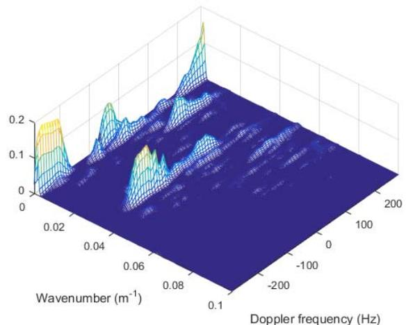
Fig. 5. PSD over spatial wavenumber and Doppler frequency, for HH polarization looking up swell.
