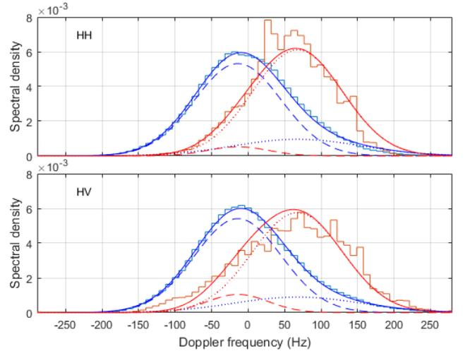
Fig. 2. Doppler (blue) and variance (red) spectra, for HH and HV polarizations looking up swell, fitted to two Gaussian components. Staircase plots, data; solid curves, overall fit; dashed curves, Bragg component; dotted curves, fast scattering component.
