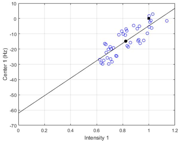
Fig. 10. Correlation between the center frequency and intensity of the Bragg component, HH polarization looking upswell. The black dot shows the mean Doppler and intensity of the Bragg component. The black square shows the arbitrary zero position of the Doppler frequency scale at a normalized intensity of 1.
