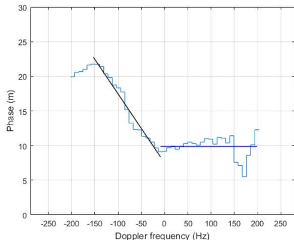
Fig. 6. Relative phase of peak intensity across the Doppler spectrum, for HH polarization looking upswell. Black regression line indicates the varying phase in the Bragg component. Blue line shows the constant phase for the fast scattering component.
