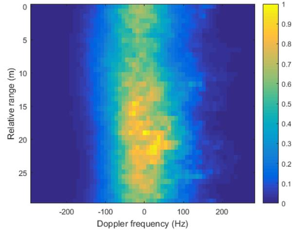
Fig. 8. Range-Doppler image for HH polarization looking up swell, averaged in range on a 30 m cycle.
