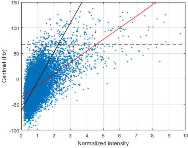
Fig. 7. Correlation between the Doppler spectrum centroid and intensity, for HH polarization, looking up swell. The red line is a least squares fit to the data. The black solid line shows the correlation between the center frequency and intensity of the Bragg component and the dashed line indicates the mean center frequency of the fast component.
