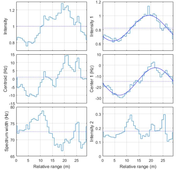
Fig. 9. Left, top to bottom: Intensity, centroid and width from the average Doppler spectrum over one swell wavelength, shown in Fig. 8. Right, top to bottom: Intensity and center frequency of the Bragg component and intensity of the fast component, calculated from the overall intensity, centroid and width using the method and assumptions described in the text. Dotted blue lines indicate the average in each plot. Blue curves are sinusoids fitted to the data.
