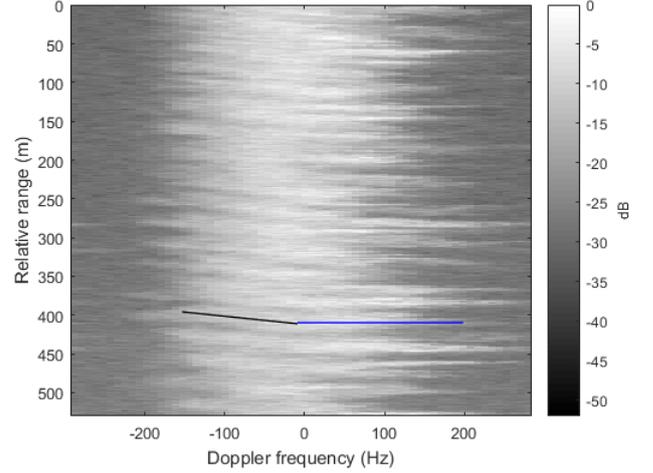
Fig. 1. Range-Doppler image for HH polarization looking up swell, averaged over 18 CPIs. Black and blue lines indicate the range-Doppler variation of the peak intensity for the Bragg and fast scattering components respectively.
