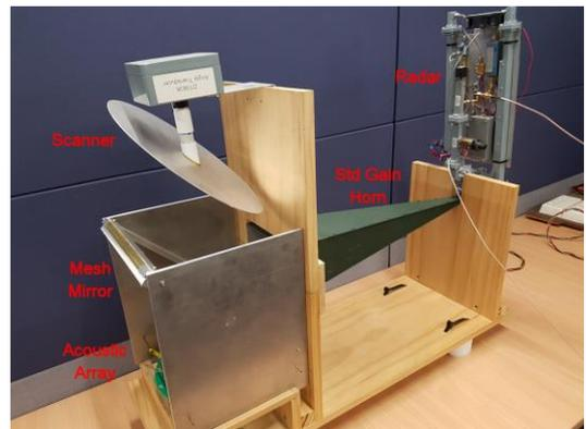
Fig. 11. Photograph of the scanning RASS sensor with the various components labelled
