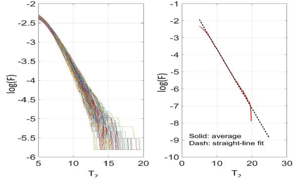
Fig. 3 False alarm curves of the A-C DF-map detector obtained using a CA sliding-window detector. Case  $L=40$  and  $F_1=0.01$ .
