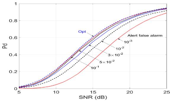
Fig. 6 Detection probability of the sequential detector at an overall false alarm rate of  $10^{-6}$  with different alert false alarm rates.
