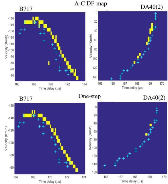
Fig. 8 Detection of targets B171 and DA40(2) versus ground truth. Rectangular dots: detections; plus signs: ground truth.
