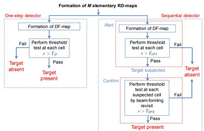
Fig. 1 Sequential A-C DF-map detector versus one-step detector.
