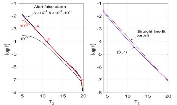
Fig. 4 False alarm curves of the A-C DF-map detector obtained using a CA sliding-window detector. Case  $L=40$  and  $F_1$  within  $[10^{-3}, 10^{-1}]$ .
