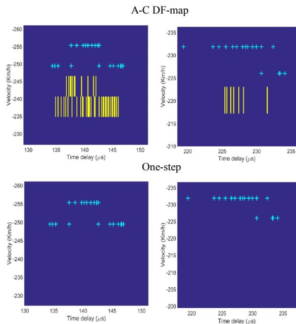
Fig. 9 Detection of targets DA40(1) and DA40(3) versus ground truth. Rectangular dots: detections; plus signs: ground truth.
