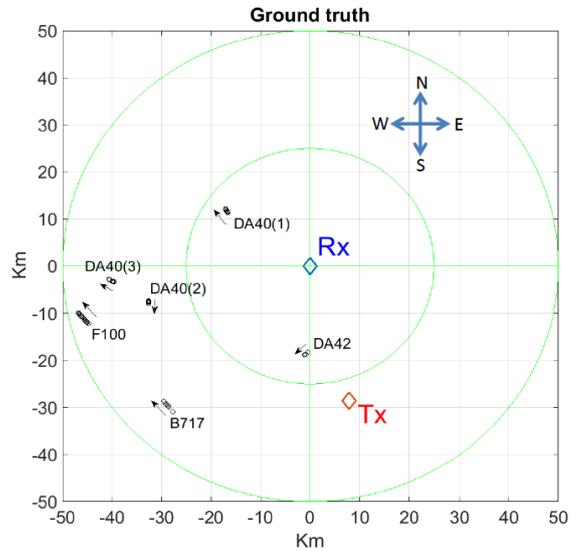
Fig. 7 The ground truth of target scenario. Rx: receiver; Tx: transmitter.
