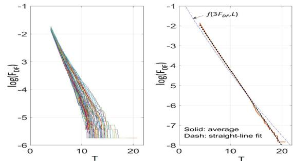
Fig. 2 False alarm curves of the one-step detector obtained by applying a CA sliding-window detector (with 40 reference cells) on the DF-map.
