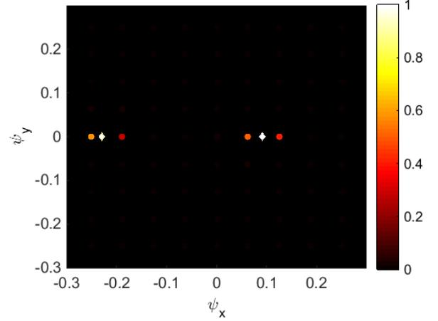
Fig. 3: Scatterers and atom intensities in  $\psi_x$ - $\psi_y$  domain for  $d = 5\lambda$
