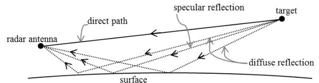
Fig. 1: Multipath propagation scenario.
