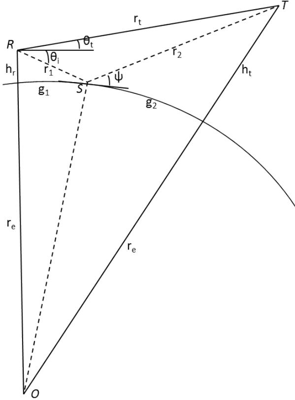
Fig. 2: Geometry of multipath propagation.
