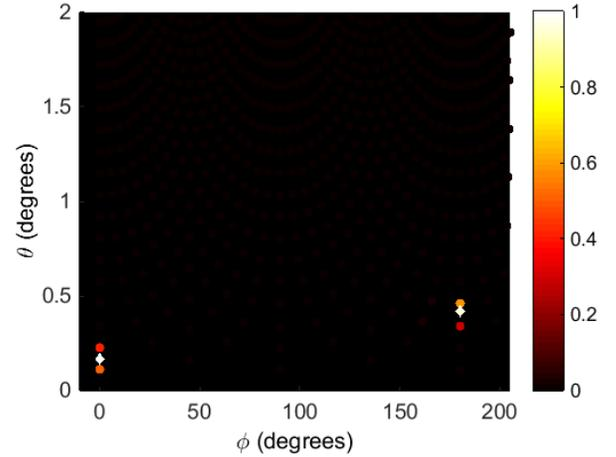
Fig. 4: Scatterers and atom intensities in  $\theta$ - $\phi$  domain for  $d = 5\lambda$
