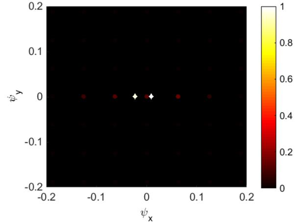
Fig. 5: Scatterers and atom intensities with element spacing of  $\lambda/2$
