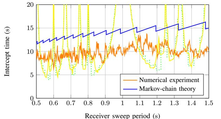
Fig. 4. Intercept time for a periodic receiver with the shuffle-scheduled BWW radar and a CTMC-controlled radar. (Light yellow and green plots are repeated from Figure 3.)
