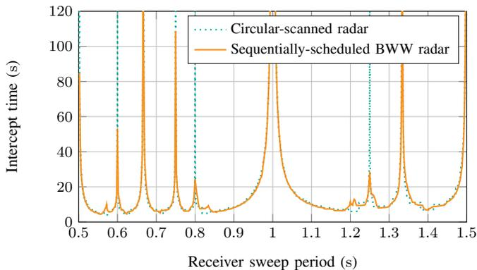
Fig. 3. Intercept time for a periodic receiver with the sequentially-scheduled BWW radar and a circular-scanned radar.
