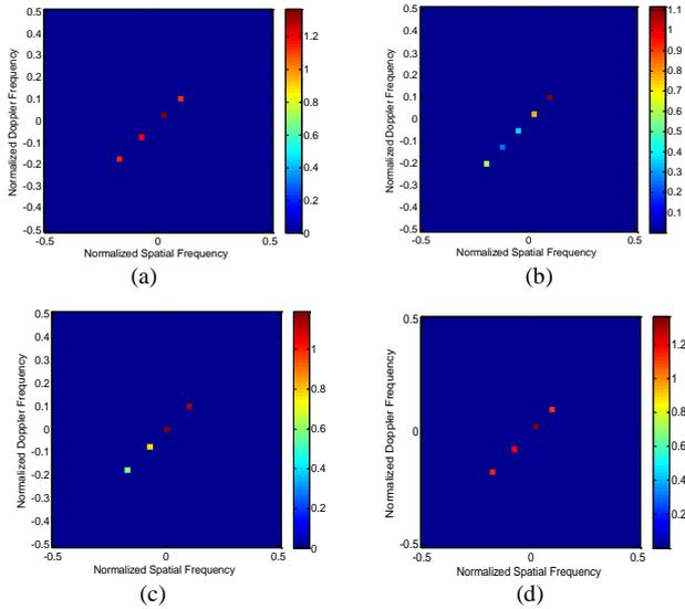
Fig. 2. Normalized spatial-temporal spectrum estimation.(a) the original clutter (b) L1-norm STAP estimation with  $KK=256$  grids (c) L1-norm STAP estimation with  $KK=1024$  grids (d) DANM-STAP estimation.
