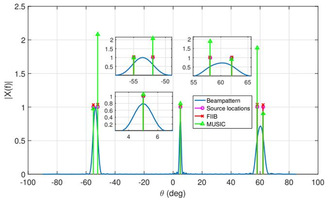
Fig. 4: Spectrum for FIIB and Root-MUSIC for the coprime pair  $M = 5$  and  $N = 7$ , with sources located at  $-55^\circ$ ,  $-52^\circ$ ,  $5^\circ$ ,  $58^\circ$  and  $62^\circ$  for SNR = 0 dB.
