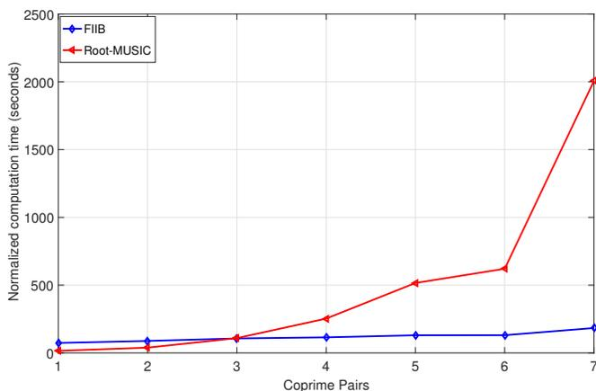
Fig. 5: Comparison of computational complexity for FIIB and Root-MUSIC for the different coprime pairs shown in Table I.
