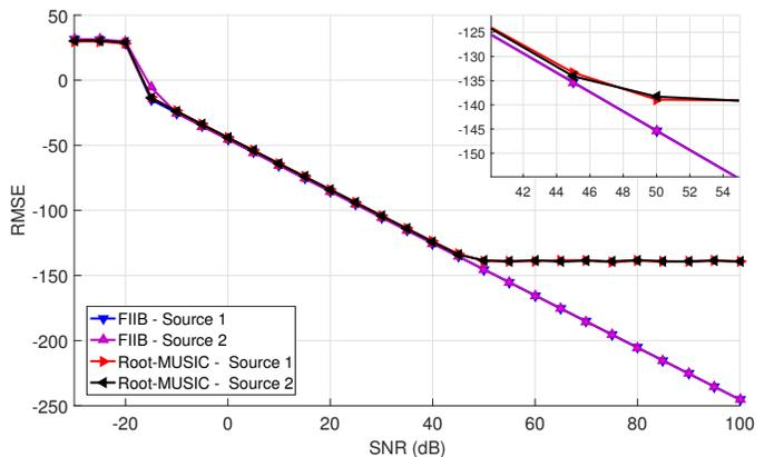
Fig. 3: RMSE of FIIB and Root-MUSIC for the coprime pair  $M = 5$  and  $N = 7$  for two sources randomly distributed along the azimuth.
