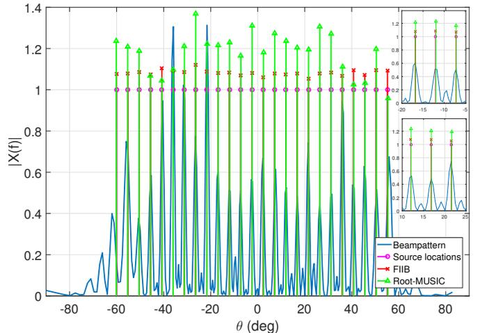
Fig. 2: Spectrum for FIIB and Root-MUSIC for the coprime pair  $M = 5$  and  $N = 7$ , with  $Q = 25$  sources embedded in SNR = 0 dB noise.
