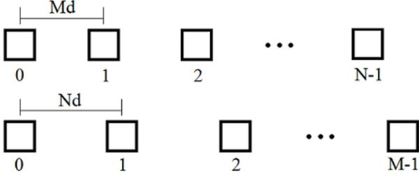
Fig. 1: The conventional coprime array configuration [16]. The first element in both sub-arrays is shared.
