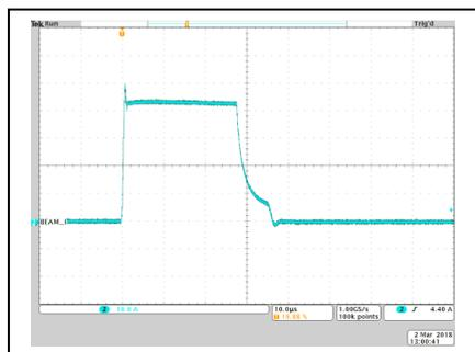
Fig. 3. Oscilloscope trace of a 30 us current pulse.
