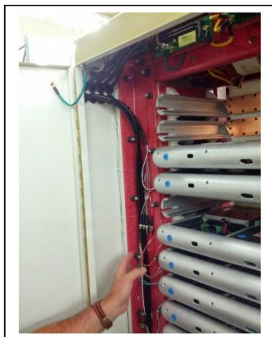
Fig. 2. Marx switch modules inside the cabinet.
