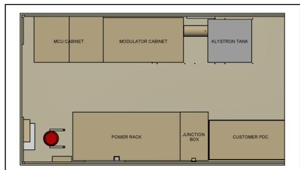
Fig. 1. Outline drawing showing the four main components of the solid-state modulator.
