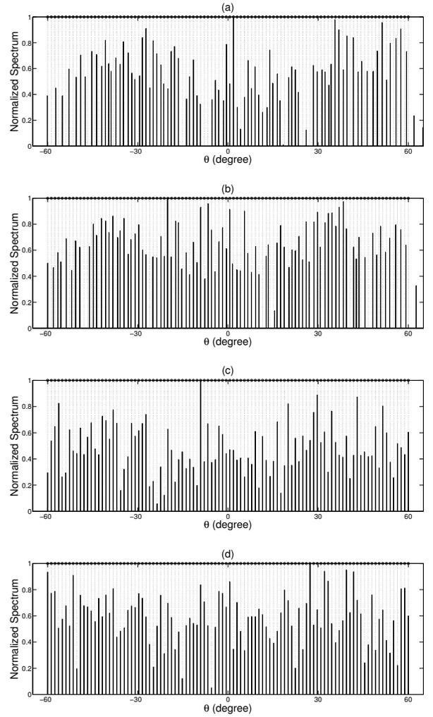
Fig. 2: DOA estimation for different NLA structures. Results for (a)FOCA, (b)FONA, (c)G-FODC<sub>NA</sub> and (d)G-FODC<sub>MRA</sub>.
