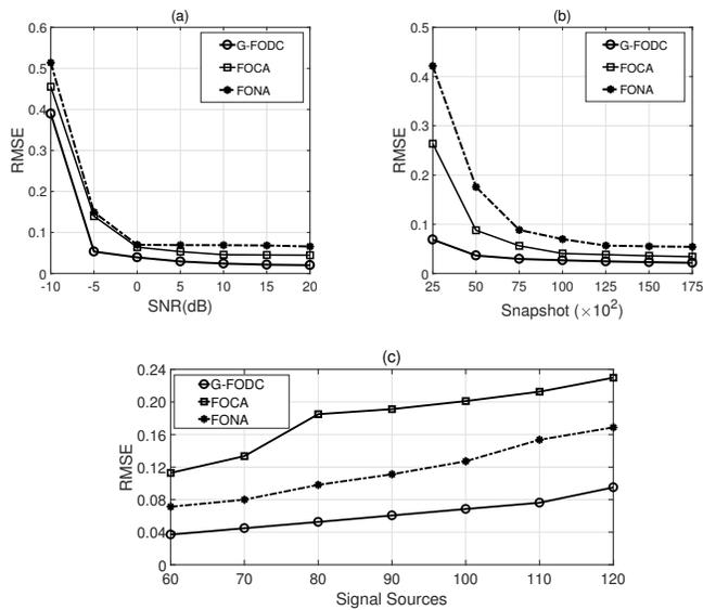
Fig. 3: RMSEs with input SNR, snapshot number and signal source. (a) versus input SNR. (b) versus the number of snapshots. (c) versus signal sources.
