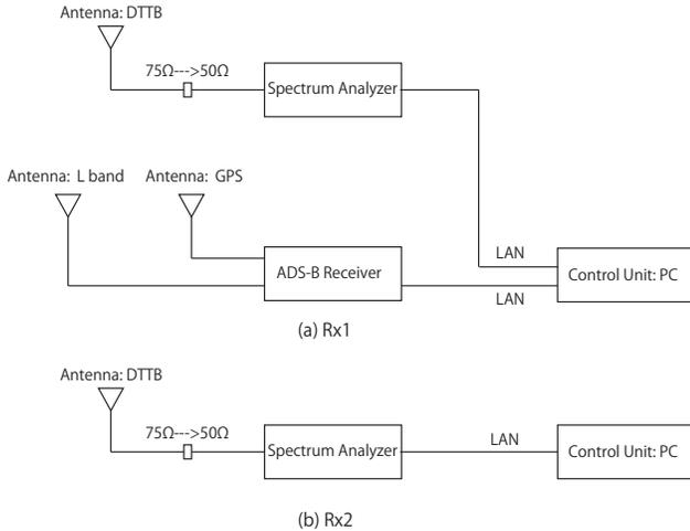
Fig. 6: A concept of MSPSR using DTTB signal delays.
