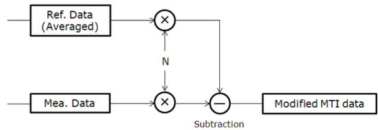
Fig. 4: Modified MTI procedure.
