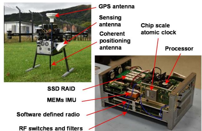
Figure 3. Functional and physical design of the sensor payload alongside the sensor integrated onto the aircraft
