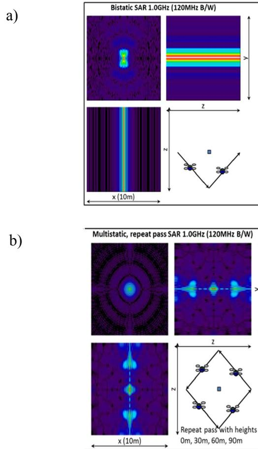
Figure 2. Transition from 0.1x0.6,m 2-D to 0.1x0.1x0.6m 3-D resolution through measurement diversity (2-D principal axis slices through 3-D image impulse responses)
