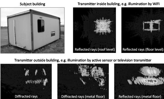
Figure 4. Computer modelling results showing building structure sensors in the measurement surface, predicting signal data. Example output from the computer modelling for a simple prefabricated building is shown in Fig 4.
