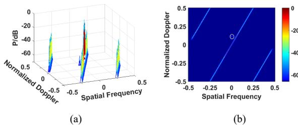
Fig. 6. Feature blocks generated in Doppler-angle domain for airborne radar (a) 3-D plot; and (b) 2-D plot.
