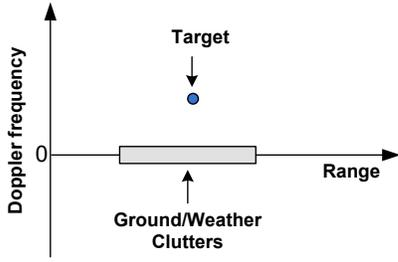
Fig. 1. Clutter and target features for MTI/MTD radars
