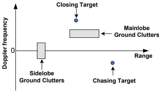
Fig.2. Clutter and target features for airborne PD radars
