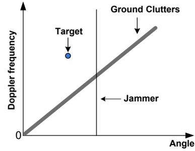
Fig. 3. Clutter, jammer and target features in angle-Doppler domain for airborne adaptive radars
