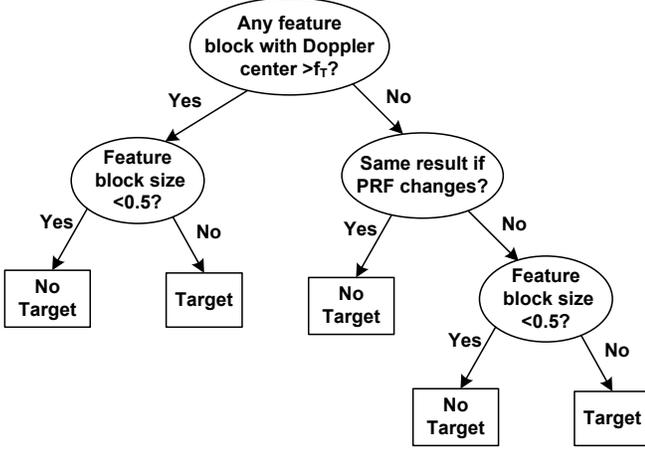
Fig. 5. A decision tree for feature-based target detection with MTI/MTD radars
