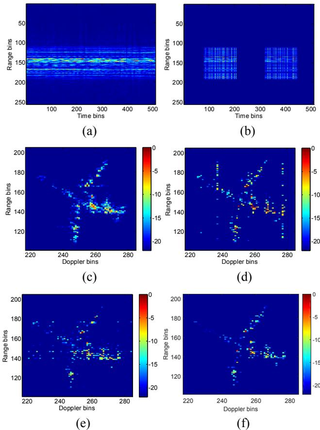
Fig. 3. Jamming suppression of Yak-42 plane: (a) range-compressed echoes; (b) gapped echoes contaminated by jamming; (c) RD image of (a); (d) OMP image; (e) RVM image; (f) image of the proposed method.
