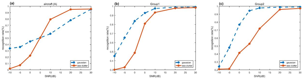
Fig. 5. Recognition rate using BP algorithm based on Gaussian and sea clutter; (a) aircraft A; (b) Group1; (c) Group2
