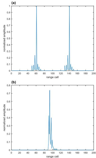
Fig. 3. (a), (b) are the simulated HRRP of Group1 with specific rotation angles; (a) is at 0 degree and (b) is at 90 degrees.
