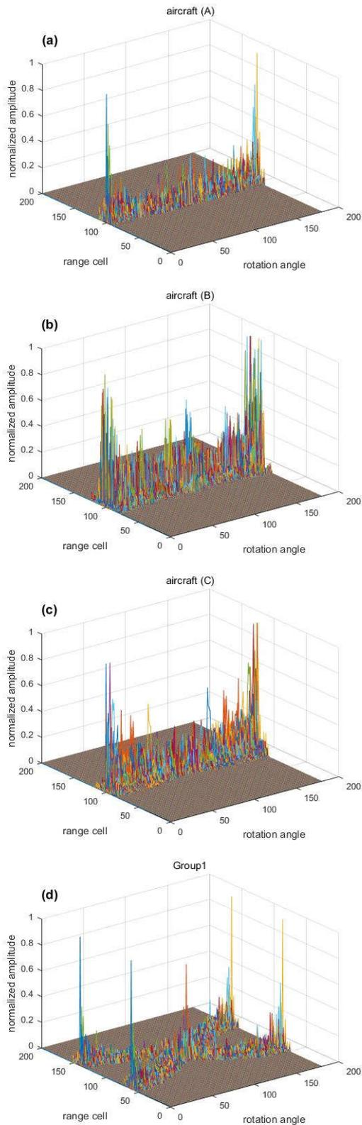
Fig. 2. (a), (b) and (c) are the simulated HRRP of three single models A, B and C respectively; (d) is the simulated HRRP of Group1; (e) is the simulated HRRP of Group2. The size of range cell depends on the actual length of the target on the LOS of radar. The radar resolution is 0.5m. Rotation angle ranges from 0 to 180 degrees. All of their amplitudes are normalized.
