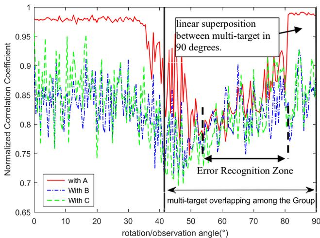
Fig. 7. Result of maximum correlation coefficient between the sample data (A, B, C) and the testing target – Group1
