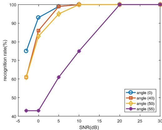
Fig. 8. Statistical recognition rate for specific single target contained in Group1 at some special angles with respect to SNR
