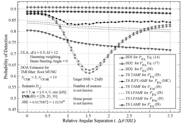
Fig. 4. Estimated probability of detection  $P_D$  versus  $\Delta\theta/SRL$ ; Scenario D2,  $m$  is not known
