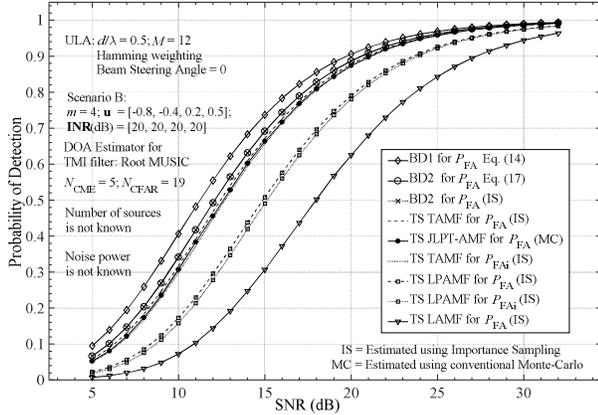
Fig. 1. ROCs for adaptive detectors under study; Scenario B,  $m$  is not known
