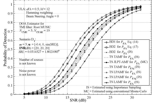
Fig. 2. ROCs for adaptive detectors under study; Scenario D1,  $m$  is not known
