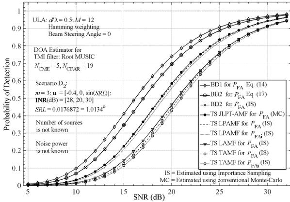
Fig. 3. ROCs for adaptive detectors under study; Scenario D2,  $m$  is not known
