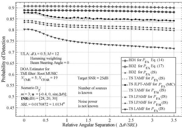
Fig. 5. Estimated probability of detection  $P_D$  versus  $\Delta\theta/SRL$ ; Scenario D2,  $m$  is known
