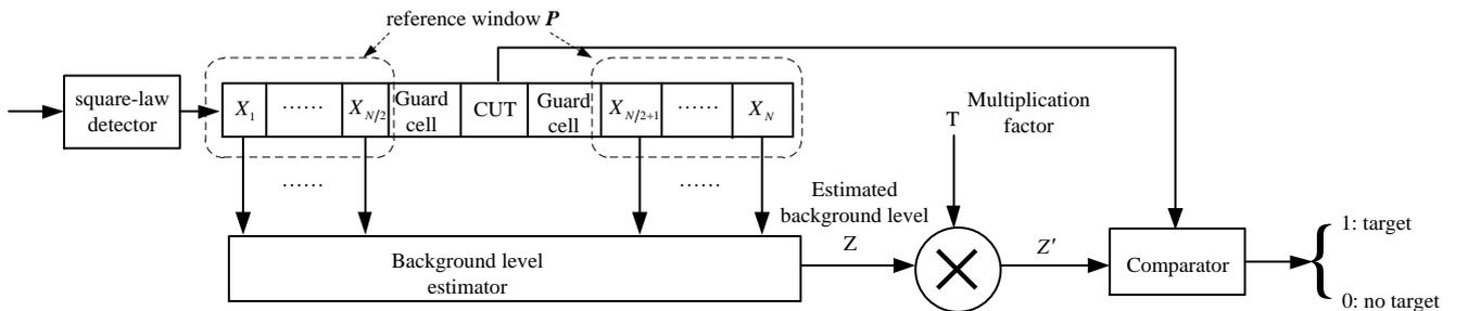
Fig. 1. Block diagram of sliding window technique.
