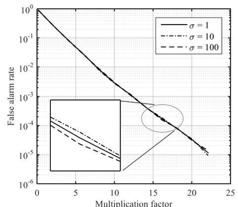
Fig. 3. False alarm rates of CAG-CFAR for different  $\sigma$  in exponential-distributed background.
