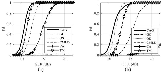
Fig. 5. Detection probabilities with (a) two interfering targets and (b) three interfering targets for ICR = SCR.
