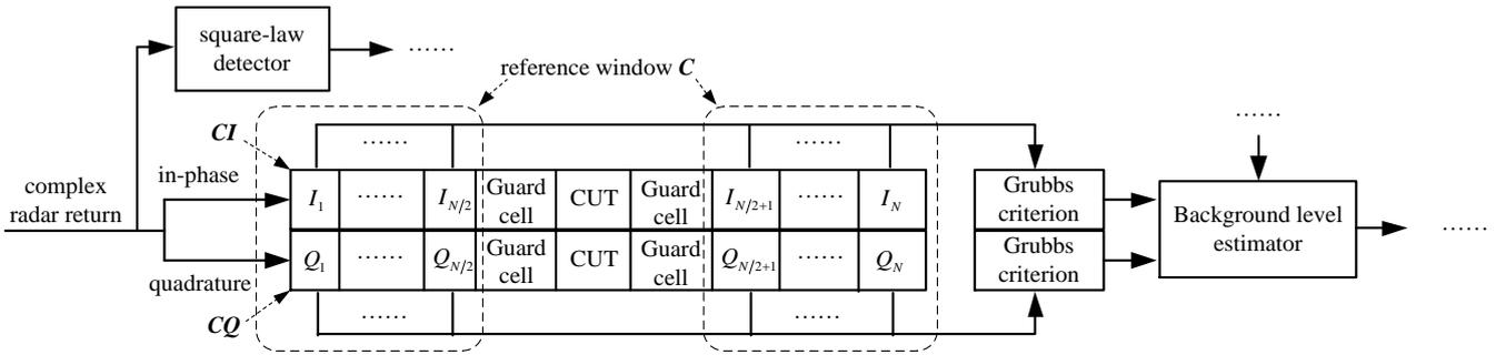
Fig. 2. Simplified block diagram of CAG-CFAR processor (omitted parts are identical to Fig. 1).
