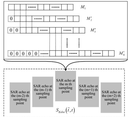
Fig.6. Echo data block handle process
