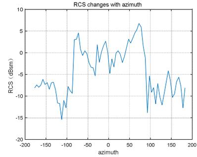
Fig.9. The change of RCS of dihedral varies with azimuth
