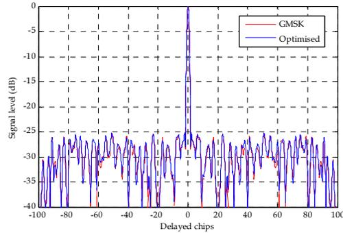
Figure 8: Pulse compressed range profiles of the original GMSK-coded QPC waveform and the optimised waveform.
