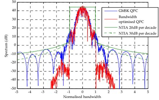
Figure 7: Comparison of the spectra of the GMSK-coded QPC waveform and the optimised waveform. The normalised bandwidth for the optimised waveform was specified from  $-1$  to  $1$ . The optimised spectrum are well within the RSEC's criteria.
