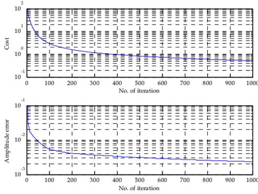
Figure 5: Both the cost and the maximum amplitude error monotonically decrease with iteration.
