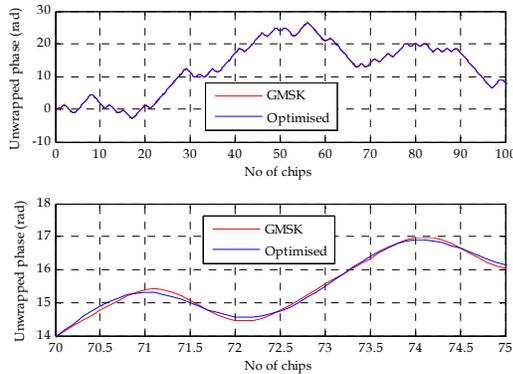
Figure 6: Two phase profiles of the initial GMSK-coded QPC waveform and the final optimised waveform. The bottom plot is a zoomed-in part of the top plot showing details of the profiles.
