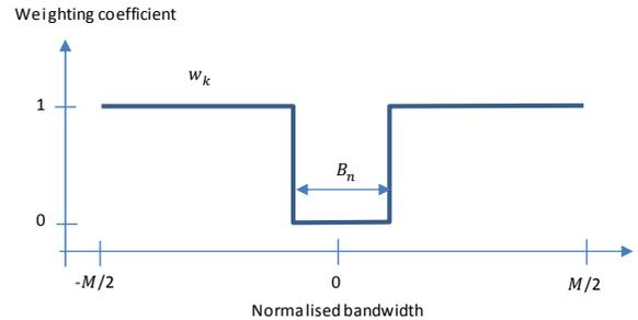
Figure 4: Weighting coefficients used in the optimisation model.  $B_n$  is the desired normalised bandwidth of the waveform. In general, the waveform is over-sampled for transmission ( $M > B_n$ ).
