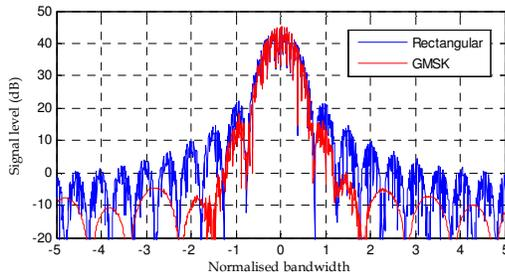
Figure 3: Comparison of the spectra of the original QPC and GMSK coded QPC waveforms ( $N = 100$ ).
