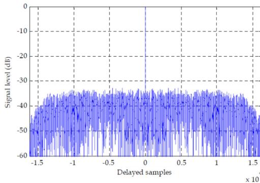
Figure 10: Autocorrelation profile of the optimised waveform composed of 3240 chips.
