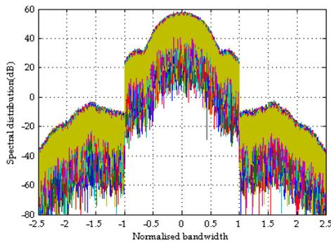
Figure 9: Spectra of 1000 waveforms. Each waveform consists of 3240 chips and each chip sampled by 5.
