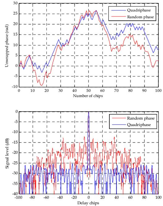
Figure 1: (top) QPC and polyphase phase profiles coded by an optimal PSL binary sequence with  $N = 100$  and  $\text{PSL} = 5$ ; (b) the corresponded autocorrelation profiles.
