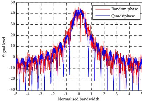
Figure 2: Spectra of the polyphase CPM and the QPC waveforms.
