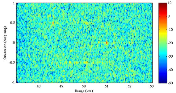
Figure 4: After pulse compression by the range-unambiguous matched filter (the current pulse) and beamforming, Targets 1 and 2 are focused and detected, and Target 3 becomes an interference signal.
