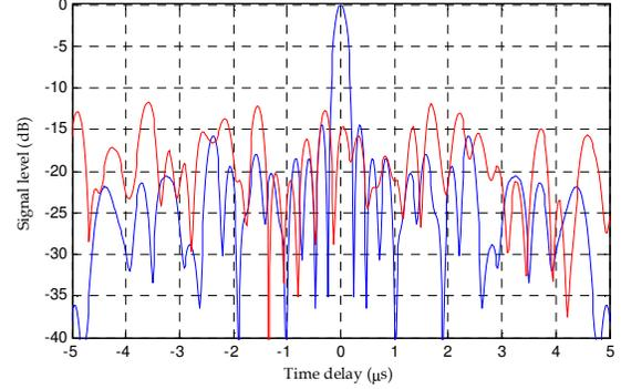
Figure 1: Autocorrelation of an FDA pulse and the cross-correlation of two FDA pulses. The waveforms are random phase coded as given by (18) ( $N+1 = 41$ ,  $T = 10 \mu\text{s}$  and  $\Delta f = 100 \text{ kHz}$ ).
