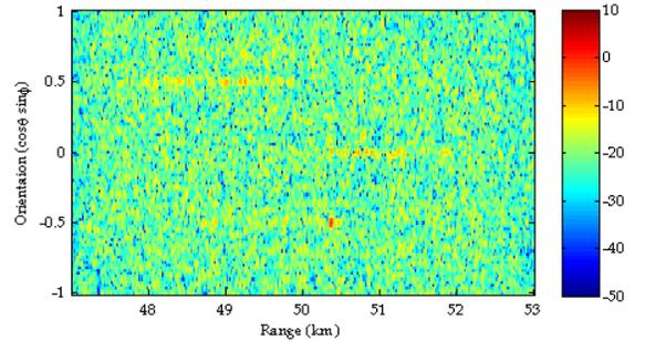
Figure 5: After pulse compression by the range-ambiguous matched filter (the previous pulse) and beamforming: Target 3 is focused and detected, and Targets 1 and 2 become interference signals.
