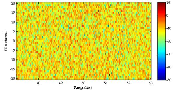
Figure 3: The simulated single-pulse received raw data in FDA channels prior to pulse compression (a noise-dominated image,  $-10$  dB SNR in raw data).
