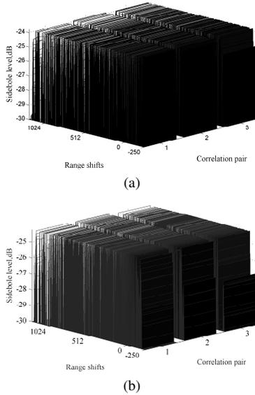
Fig. 5. (a) Cross correlation sidelobes of phase coded signals and LFM signal with longer pulse durations. (b) Cross correlation sidelobes of phase coded signals and LFM signal with longer bandwidth.
