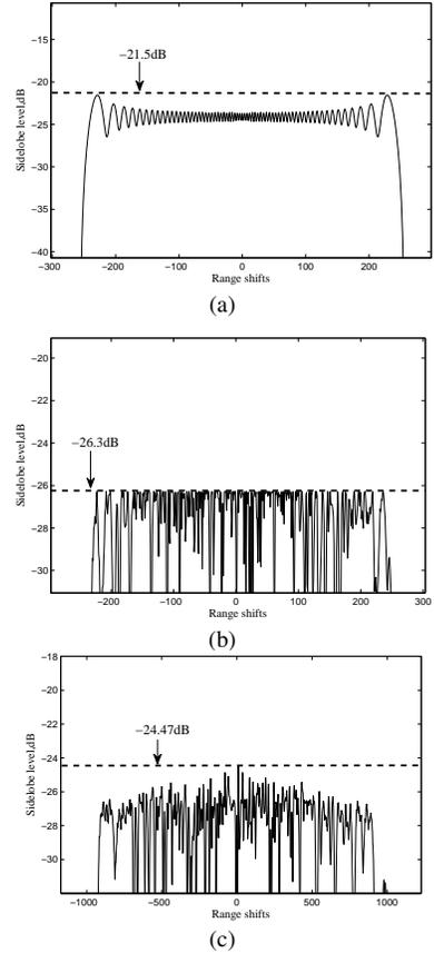
Fig. 1. (a) Cross correlation sidelobes between LFM signals with opposite frequency modulation ratios; (b) Cross correlation sidelobes between a phase coded signal and LFM signal after optimization; (c) Cross correlation sidelobes between phase coded signals and the LFM sampled at frequency 80MHz.
