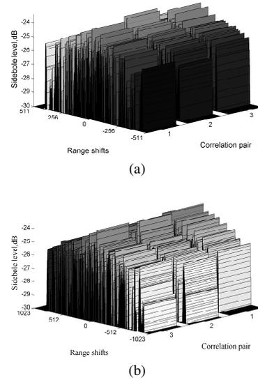
Fig. 3. (a) Cross correlation range sideboles of phase coded signals and LFM signals under double sampling. (b) Cross correlation sideboles of phase coded signals and LFM signals under 4 times sampling.
