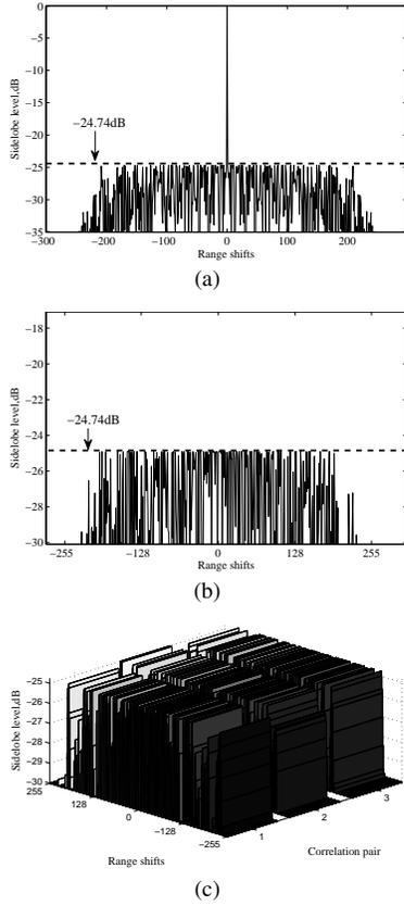
Fig. 2. (a) Autocorrelation sideboles of phase coded signals; (b) Cross correlation sideboles between phase coded signals; (c) Cross correlation sideboles of phase coded signals and LFM signal.
