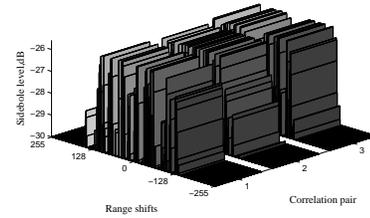
Fig. 4. Cross correlation sideboles between phase coded signals and LFM with a window.
