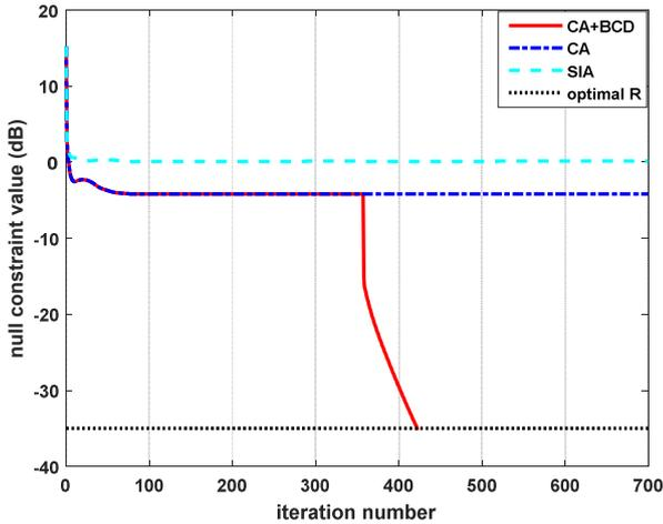
Fig. 3(a). The value of the null constraint versus iteration number.
