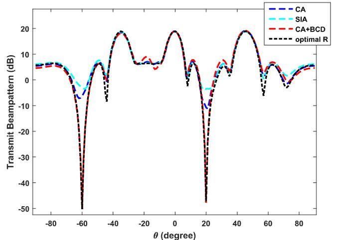
Fig. 2. Transmit beampattern of CA, SIA, CA+BCD and optimal  $\mathbf{R}$  considering the first order derivative constraint.
