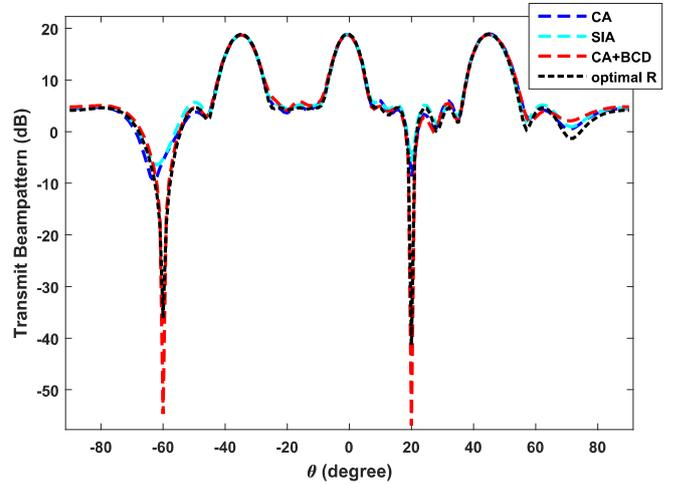
Fig. 1. Transmit beampattern of CA, SIA, CA+BCD and optimal  $\mathbf{R}$  considering the zero order derivative constraint.
