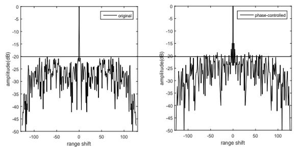
Fig. 2. auto correlation of angular waveform before and after phase disturbed
