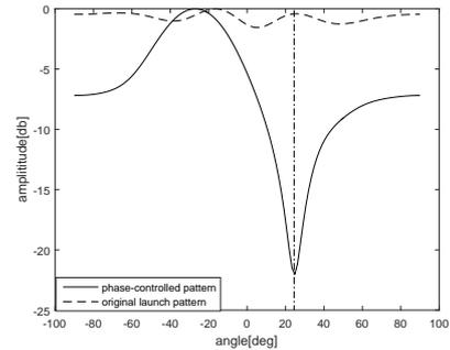
Fig. 1. transmit beampattern before and after phase disturbed
