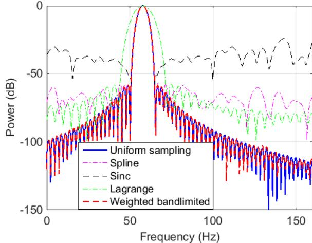
Fig. 2. Comparison of interpolation based spectral estimations of nonuniform sampled signals.
