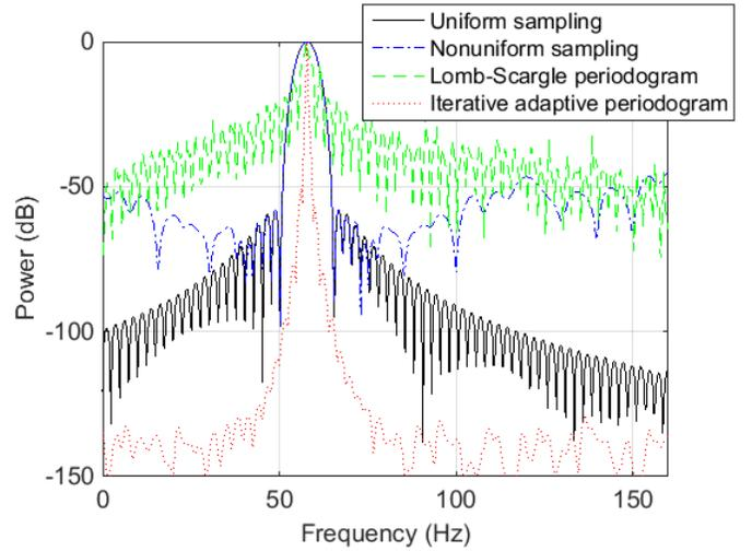
Fig. 1. DFT based spectral estimation of nonuniform sampled data with Blackman window compared with two periodogram based spectral estimations.
