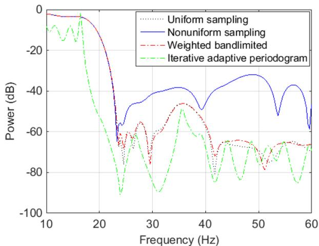
Fig. 4. Doppler spectra of nonuniform sampled signal in the presence of clutter for a Swerling 2 target.
