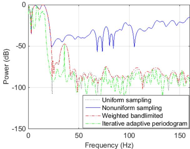
Fig. 3. Doppler spectra of nonuniform sampled signal in the presence of clutter for a non-fluctuating target.
